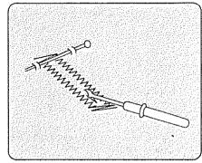
7. Remove the fabric and cut the hole open with the buttonhole opener in your accessory box.
